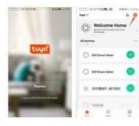
· Click "all device" and find out the "socket" item to select. Turn the power on of the power meter and long press switch for 5 seconds till the network indicator flashes rapidly, click "confirming the indicator is flashing rapidly" button.
